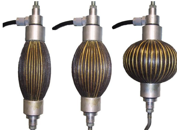
Figure 2.8: A Pleated Pneumatic Artificial Muscle from Vrije Universiteit Brussel, shown in three stages of contraction as the internal air pressure is increased.
