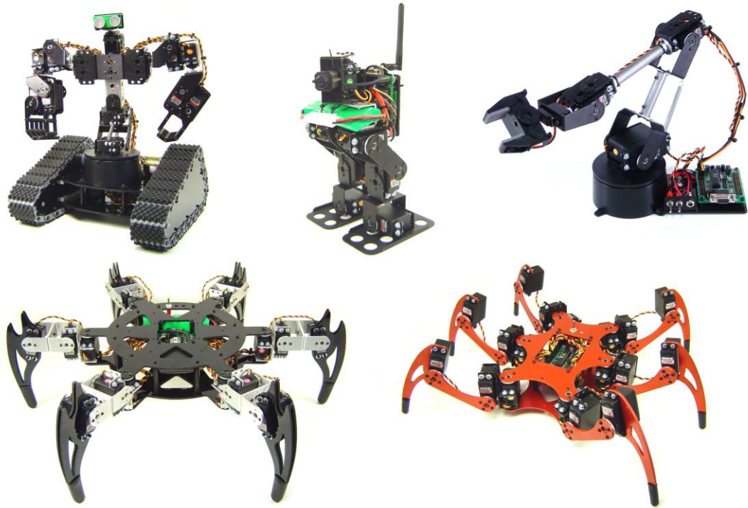
Figure 1.3: A range of small robots constructed by a company called Lynxmotion, intended for the hobbyist and all using position controlled servos.
