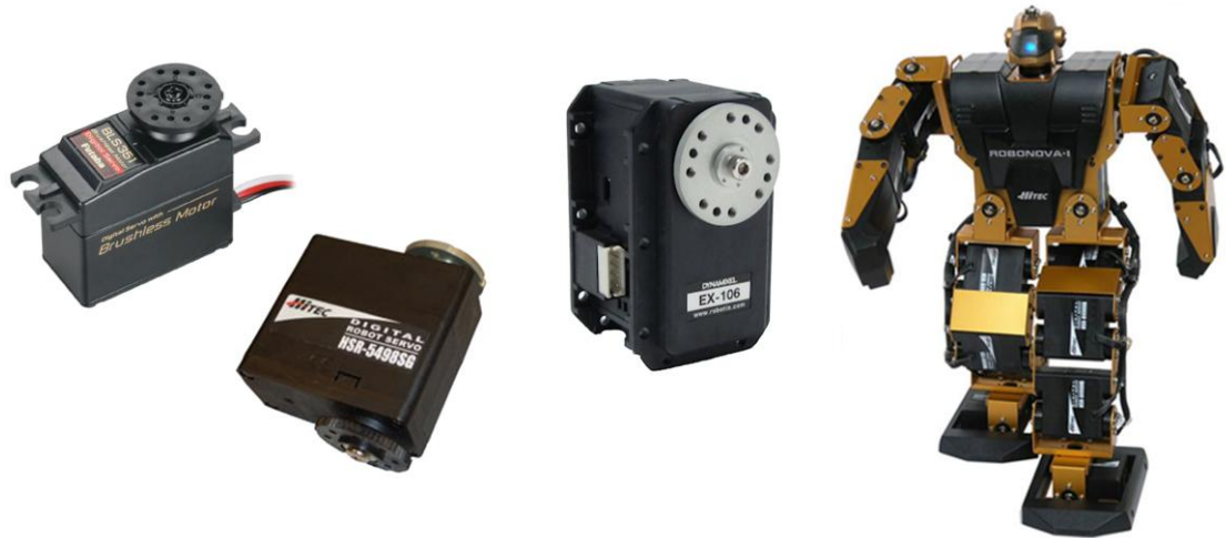
Figure 1.2: The hobby servo on the far left has recently been adapted for the emerging hobby robotics market with manufacturers producing versions of actuators specifically for robot builders, and new companies producing them specifically for these markets. The primary enhancements to these products are generally an increase in torque output and provision of sensory feedback to an external controller.
