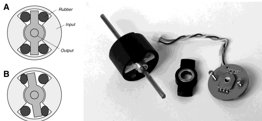
Figure 4.3: A rubber based force sensor consisting of an outer barrel and inner shaft coupled together with rubber bushes via tabs on each part of the device. Normally the rubber keeps the two parts in a central position (A) but a force difference will cause one pair of rubber bushes to compress (B). The outer part would be driven via a spur or bevel gear and transfer the torque to the output shaft via the rubber. A potentiometer can be used to measure the displacement.
