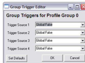
Figure 5.13: Configuring group triggers. The group trigger allows you to evaluate several flags at once and generate a true or false output if any of its inputs is true. It effectively operates as a four input OR gate.
