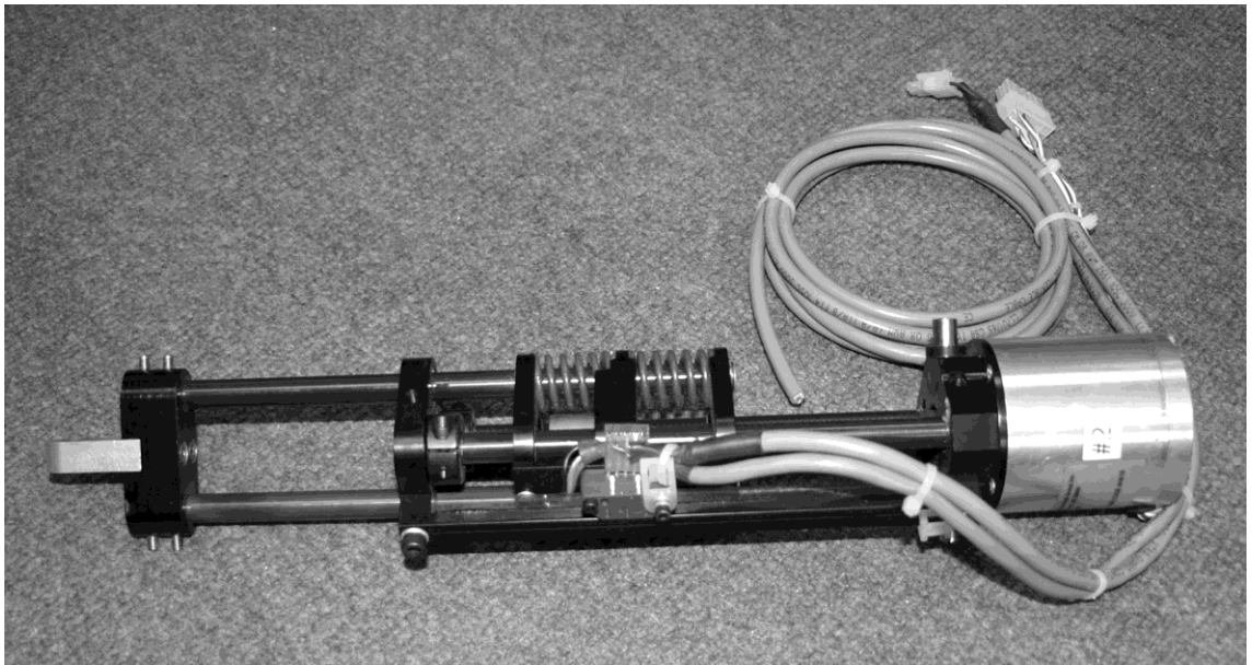
Figure 2.3: A Series Elastic Actuator made by Yobotics 1 (shown without the control electronics).
