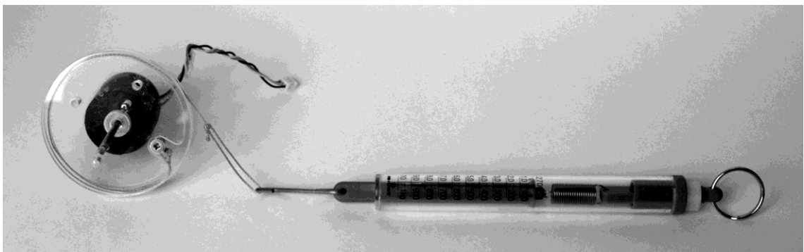
Figure 4.2: A spring weight gauge and pulley wheel attached to one of the rotary force sensors.
