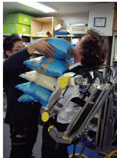
Figure 19 Lifting rice bags with the Muscle Suit, Tokyo University of Science Photo: Rinie van Est
