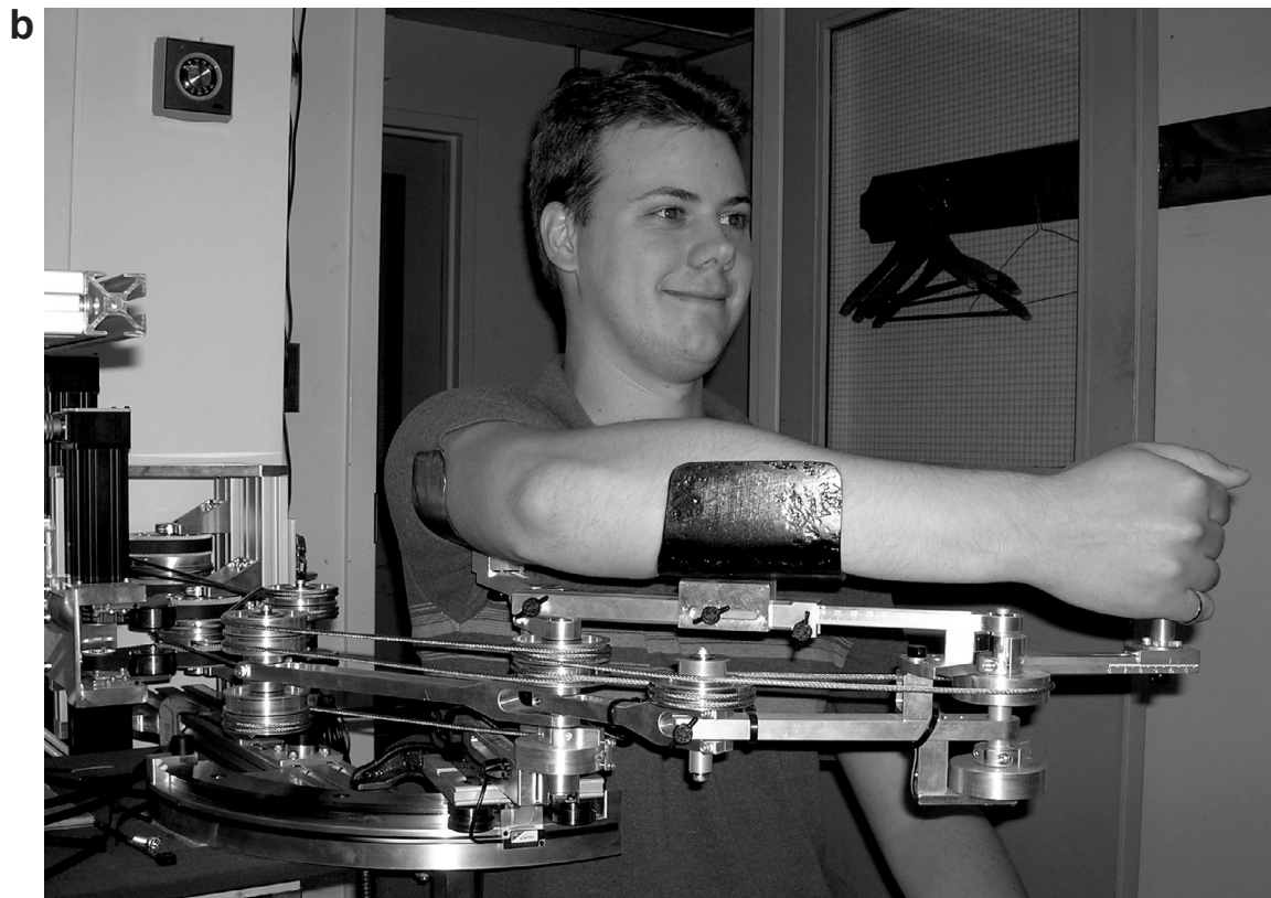
Figure 6.1: (a) A photo of the fully constructed Planar MEDARM prototype in its original configuration. The view was chosen to match the CAD view from Fig. 5.2a. (b) A photo of Planar MEDARM in use.
