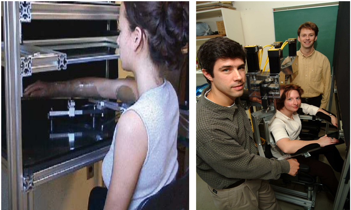
Figure 3.1 Bilateral KINARM device used in this study.
