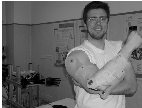
Figure 8.14 The first version of the NEUROExos
