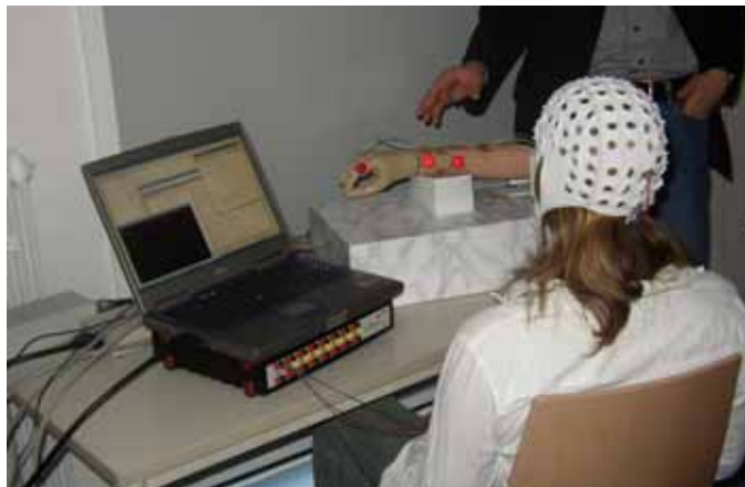
Figure B.5. Live demonstration of a mechanical arm controlled in four degrees of freedom by steady-state visual potentials. Each of the lights oscillates at a different characteristic frequency. Attending to a given light enhances EEG at that frequency and harmonics. When the BCI detects this signal, it causes the arm to move about the associated axis.
