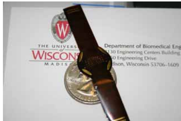
Figure 2.14. Subdural ECoG microgrid for epidural recordings (reprinted with permission from D. Moran).
