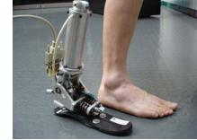
Fig. 1 A prototype of the robotic ankle-foot emulator.
