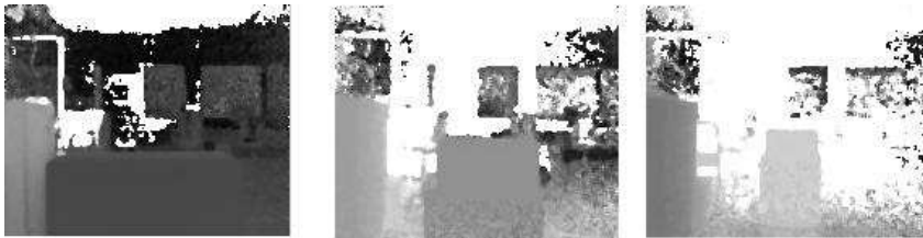
Figure 81: Depth images for different distances and a 18ms integration time.
