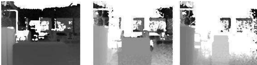
Figure 82: Depth images for different distances and a 50ms integration time.
