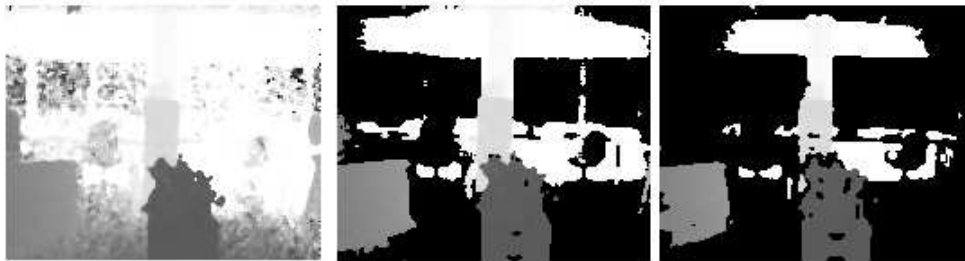
Figure 93: Highly noisy images taken using different amplitude thresholds.
