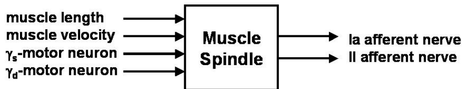
Figure 4.7: A block scheme showing the two mechanical inputs (length and velocity) and two neural inputs ( \gamma_d and \gamma_s motor neurons), and two neural outputs (Ia and II afferent nerves) of the muscle spindle.
