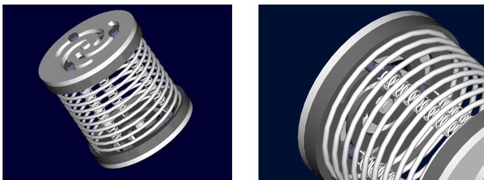
Figure 9.1: The prototype consist of three NiTi springs inside an exoskeleton, made of a spring with very low stiffness. The two covers can adjust the distance between the NiTi springs. Heating one of the NiTi springs by applying a voltage will shorten the NiTi spring and a rotation will follow
