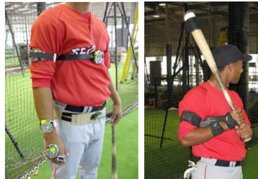
Figure 4: Nodes initially applied to player (left) and fully taped up during data taking (right)
