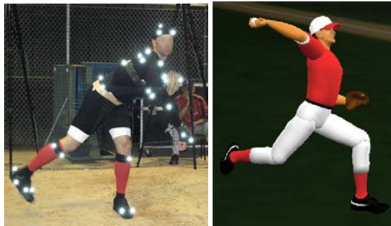
Figure 3: Setup with reference camera tracking system (top), pitcher w. targets (left) & reconstruction (right)
