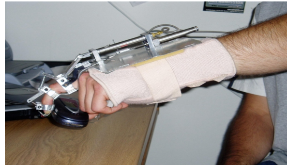
Fig. 1. Our orthotic exoskeleton system. It is a low-profile lightweight exoskeleton that allows basic pinching motion using natural sequence of muscle activation. Pinching motion between the index finger and the thumb provides the ability to perform a wide range of daily tasks.
