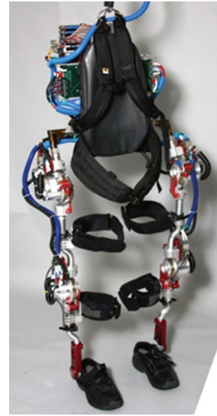
FIGURE 1: The IHMC Mina sensorimotor robotic orthosis for mobility assistance prototype. Mina adjusts to fit users ranging from \sim 1.6 m to 1.9 m tall.
