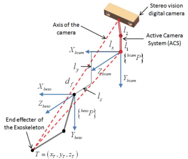
**Fig. 5.** Camera positioning for tracking the end-effector.
