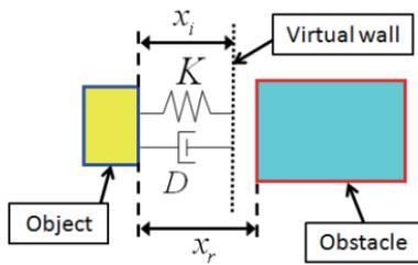
Fig. 6. Virtual wall for obstacle avoidance.
