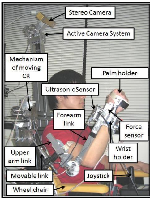
(a) 4DOF upper-limb power-assist exoskeleton robot
