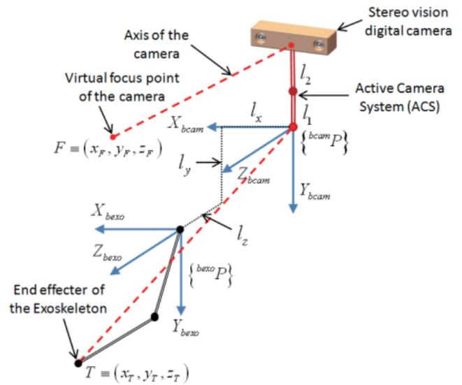
**Fig. 4.** Initial camera positioning and virtual camera focus.
