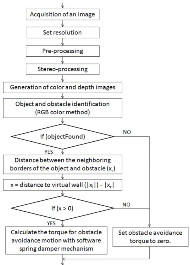
Fig. 7. Obstacle avoidance algorithm.
