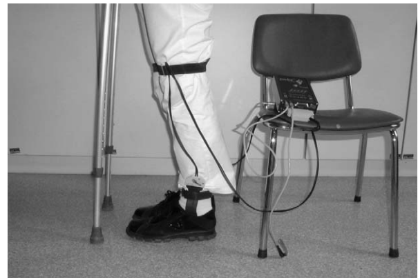
Fig. 1. A patient wearing pedar mobile system connected to a portable data set.
