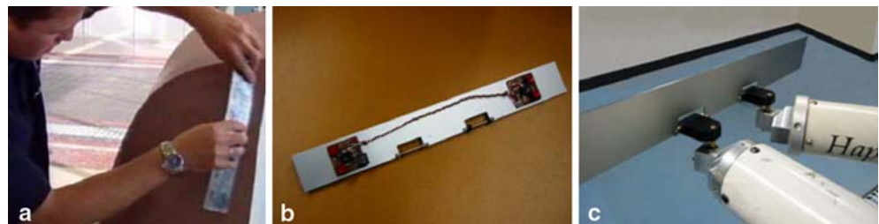
Fig. 4 Haptic virtual rake: (a) real rake used by designers for clay modeling; (b) virtual rake; (c) rake mounted on a six DOF haptic system
