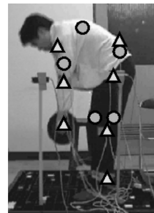
Fig. 5. Sensor location in measuring human motion. The triangular points represent three-dimensional position sensors and the circle points represent EMG electrodes.
