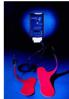
(b) Novel Pedar insole pressure sensing system.
