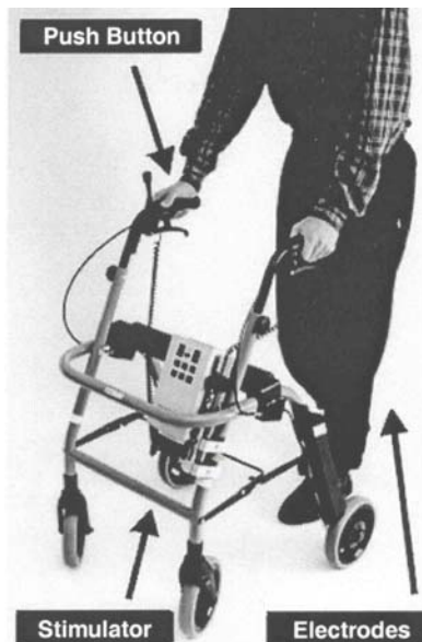
Figure 2.17 ETHZ-Paracare push button drop foot system (Popovic, 2001).
