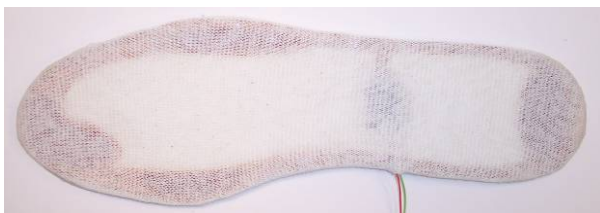
Fig. 8. The ACHILLE interface is a wireless control interface that can be inserted inside the shoe and can be used to control external devices.
