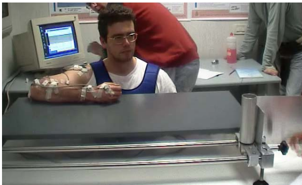
Fig. 1. Ad hoc catching platform during tests on a subject. On the right side of the figure the handle (target) is placed on a slider. The slider runs on two bars by means of two linear bearings. A spring mechanism push the slider that is release unexpectedly by the tester.
