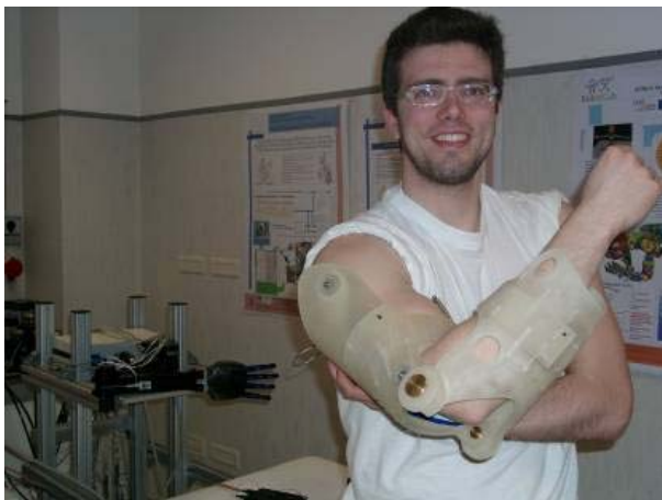
Fig. 5. Rapid prototyping mock-up of the NEUROExos elbow module.
