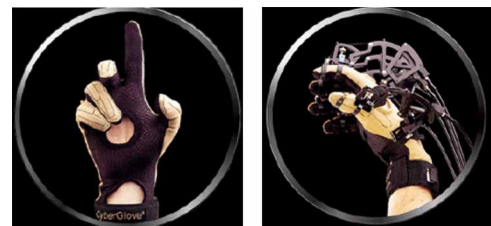
Fig. 3 The CyberGrasp exoskeleton-type system [21]
