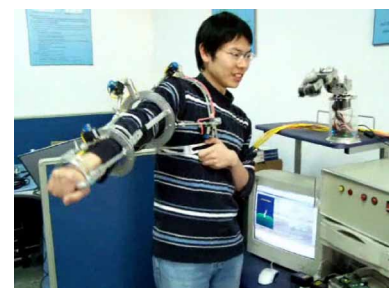
Fig. 4 The six-degree-of-freedom ZJUESA exoskeleton system
