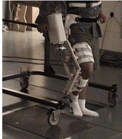
Fig. 4. Engineering prototype mounted on the walking frame and the subject in the gravity-balancing device.
