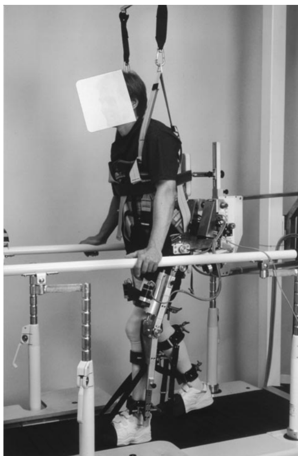
Figure 1 Illustration of a patient with incomplete paraplegia during an automated locomotor training with the DGO
