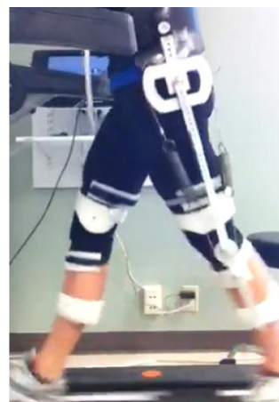
Figure 1. We built a passive exoskeleton with two-joint springs crossing the hip and knee. The design of this device was based on previous model simulations, with the goal of providing swing phase gait assistance.
