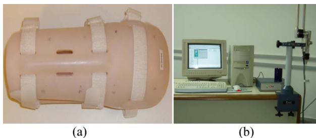
Fig. 2. (a) The plastic humeral splint with the holes on top of it (black dots), (b) Experimental setup consisting of the FARO IND-01 CMM arm placed on the right and the corresponding software for data acquisition.
