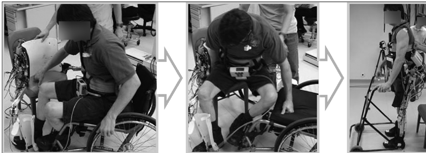
Figure 3. Subject donning hybrid neuroprosthesis.
