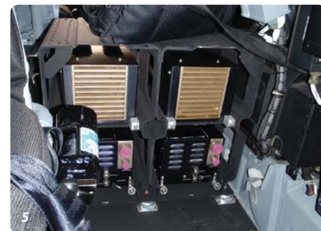
5 Cobham Microclimate Cooling Units (4) installed on Blackhawk helicopter
