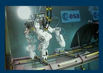
The goal of the project was the realization of EWM (Eurobot Wet Model), an in-water test-bed of the Eurobot system which will be used on the ISS (International Space Station) as a robot servant for performing Extra-Vehicular Activities.
