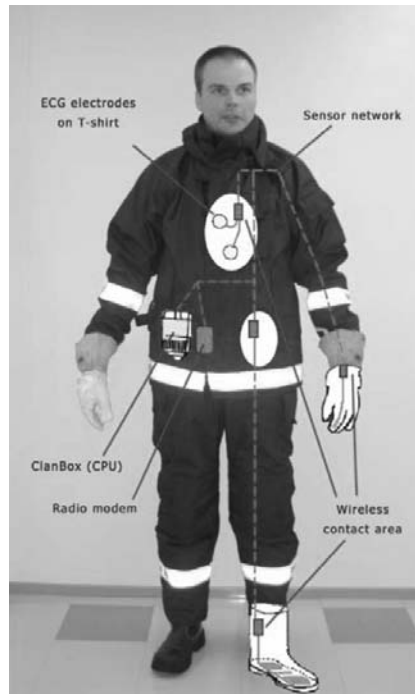
Figure 7.6 The structure and components of the CLAN prototype system
