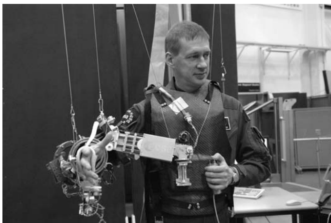
Figure 8.8 The ESA ergonomic exoskeleton worn by ESA Astronaut Frank de Winne during an evaluation session. Reproduced from ESA
