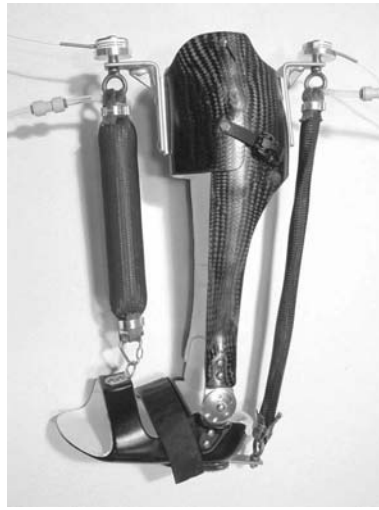
Figure 9.5 Ankle–foot orthosis. The shank section is made from carbon fibre and the foot section is made from polypropylene. The artificial dorsiflexor muscle is fully inflated and the artificial plantar flexor muscle is relaxed for comparison. Artificial muscle tension is monitored by load sensors in series with the artificial muscles
