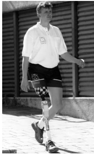
Figure 6.17 A Prolite™ Smart Magnetix™ above-the-knee (AK) prosthesis user walking down a slope: the characteristics required for the knee prosthesis will generally be different from other walking conditions. The MR technology provides the desired adaptation. Reproduced from Pons 2005
