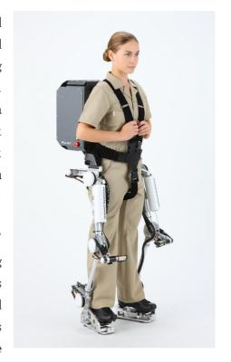
motion of the operator legs and producing an augmentation of leg strength. According to current specifications, this augmentations can go up to 40kgf (around 400N)
