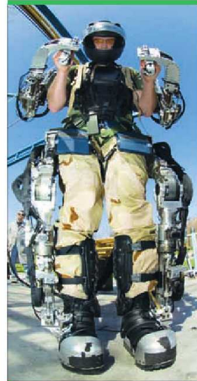
Raytheon's purchase of Utah-based Sarcos has given the company a portfolio of exoskeleton expertise. The firm's Xos is expected to be developed as a prototype suit for the US military to assist logistical tasks. (Raytheon)
