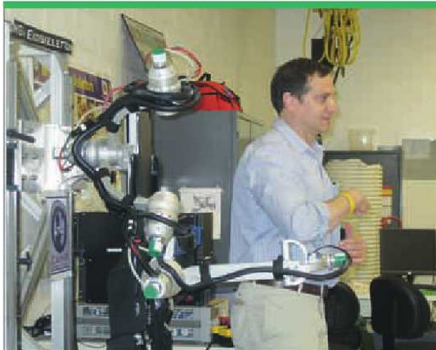
Several exoskeleton projects are ongoing in the academic and civilian worlds, which could develop technology that could be spun out into military applications, such as this University of Maryland's Exoskeleton Rehabilitation System. (University of Maryland)
