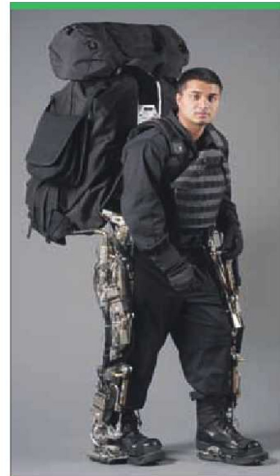
The University of California's Berkeley Department of Mechanical Engineering has developed the Bleex (Berkeley Lower Extremity Exoskeleton) machine which was the result of Darpa funding. (University of California)
