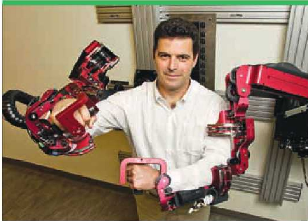
Several academic institutions are performing important research into powered exoskeletons. One such project is being pursued by the University of California's Baskin School of Engineering, which has developed a set of prototype exoskeleton arms. (BSE/JM)
