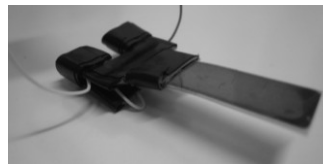
Fig. 1. An Electroactive Polymer Actuator
