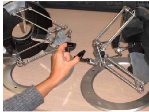
Figure 5: Two Omega devices were used in [18] for 3D real-time haptics interaction.
