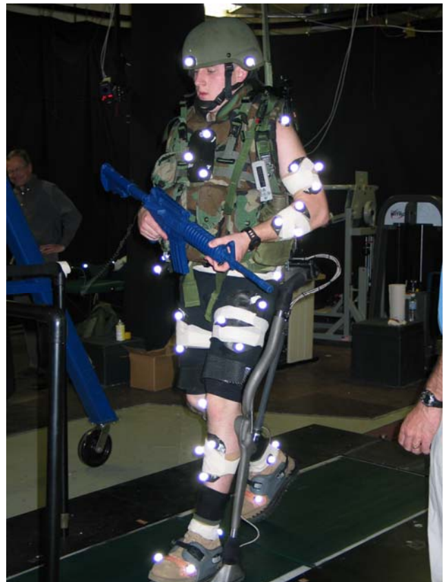
Fig. 2. Soldier wearing EXO prototype and fighting load with retro-reflective markers placed for motion capture collection.
