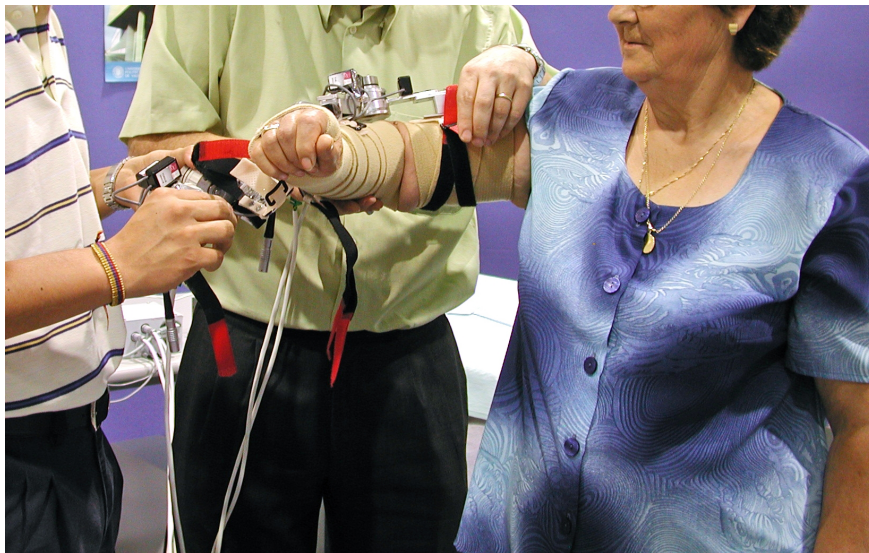
Fig. 5.1 Illustration of the process of placing WOTAS over the arm of a patient during experiments.
