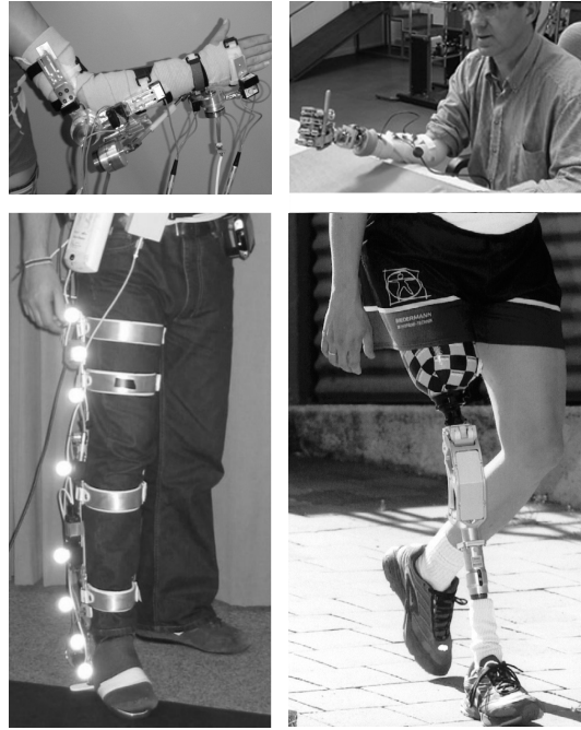
Fig. 1.1 Wearable robots: (top left) an upper limb orthotic exoskeleton; (top right) an upper limb prosthetic robot; (bottom left) a lower limb orthotic exoskeleton; (bottom right) a lower limb prosthetic robot.
