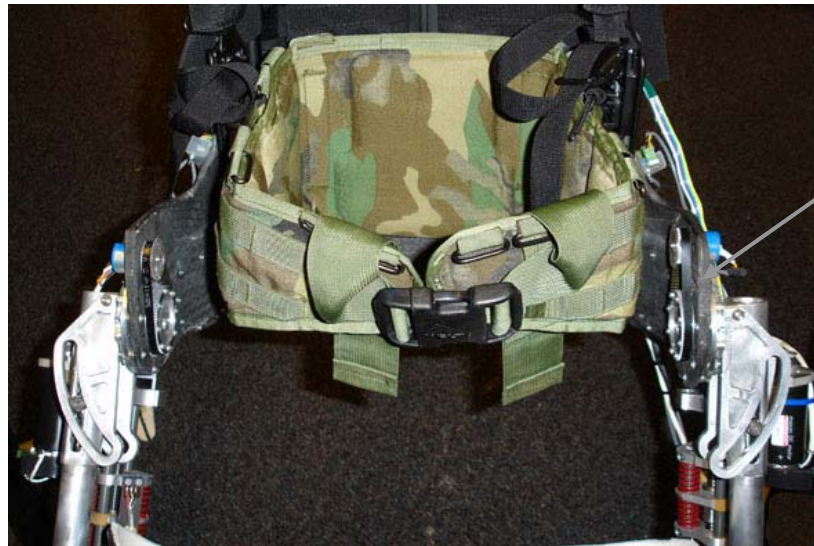
Figure 4.5 Hip angle sensing was done by means of a timing belt and pulley with a 2:1 reduction on a Bourne's rotary pot. The belt system was attached to the hip joint on the inside of the harness as shown.
