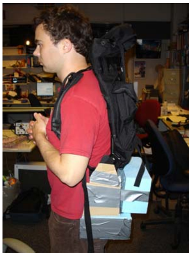
Figure 3.4 Foam mockup of the exoskeleton harness being tested.
