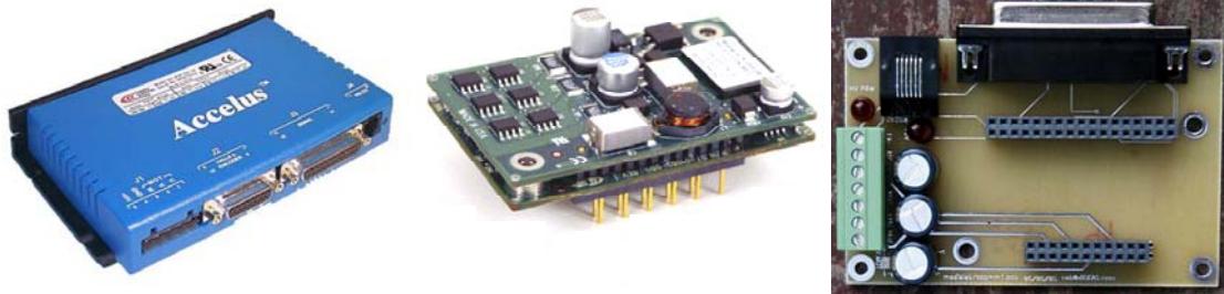
Figure 4.2 In a), the Accelus digital amplifier used at the hip is shown. In b), the PCB mount Accelnet micro-module used at the knee required a breakout board. In c), the custom breakout board for the Accelnet
