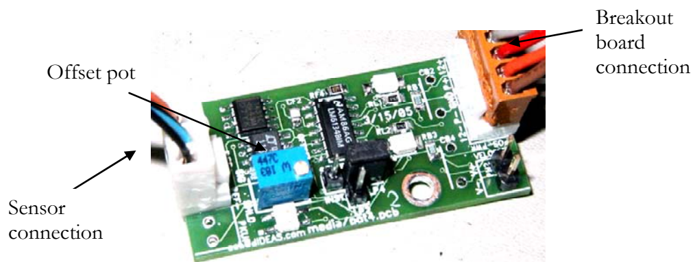
Figure 4.3 Signal conditioning board. One side reads in the voltage from a strain gauge bridge or potentiometer. The other connector differential power to the board and sends an amplified differential signal to the breakout board that gets read by the D/A board.
