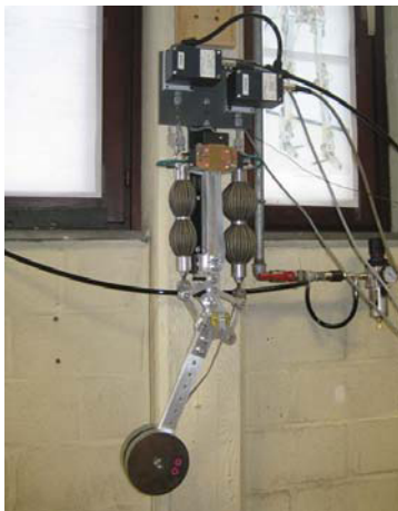
Fig. 3. Simplified 1 DOF test setup for control evaluation
