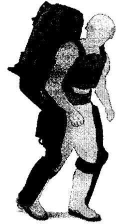
Fig. 1-1 Illustration of the Berkeley Lower Extremity Exoskeleton (BLEEX) from the 2004 New York Times: Year in Ideas [1]
