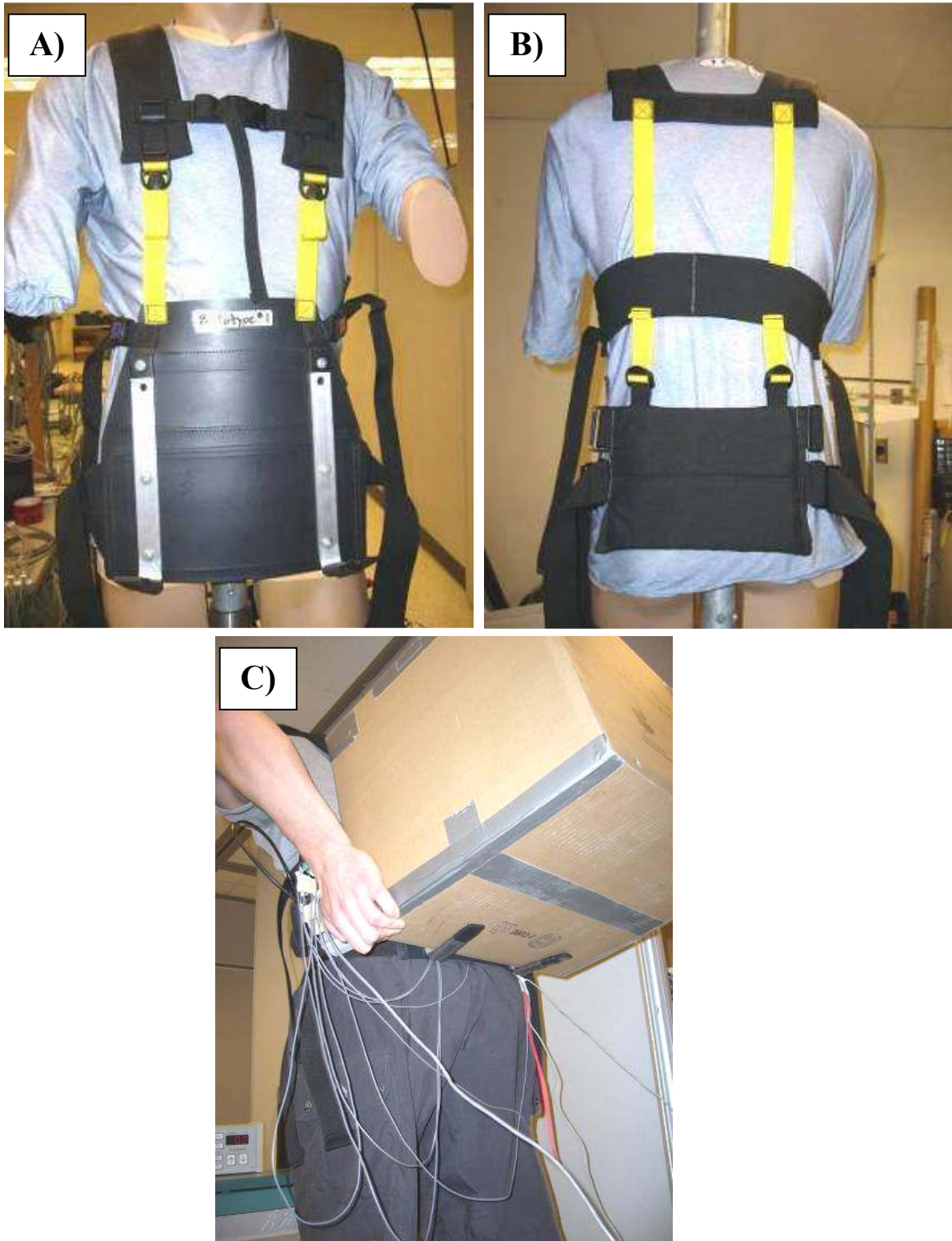
Figure 5.1 – Photographs of the assistive device used in this study. Part A) displays the side of the assistive device that articulates with the load being carried. B) displays the harnessing that secures the device to the body. C) Shows the device being used by a subject during PCD. Note how the aluminum stays project outward from the lower sacrum to support the vertical force component of the load
