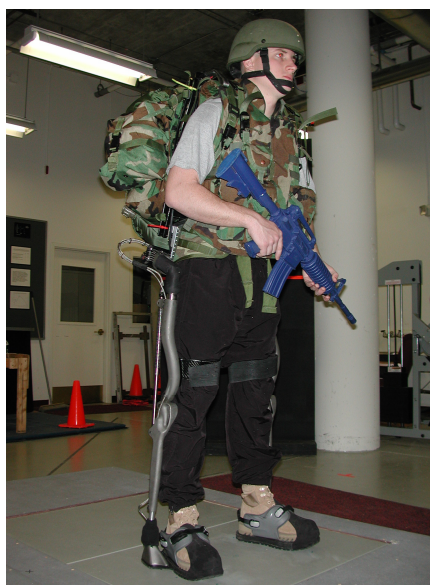
Fig. 1. Soldier wearing EXO prototype and emergency approach march load, while standing on force plate
