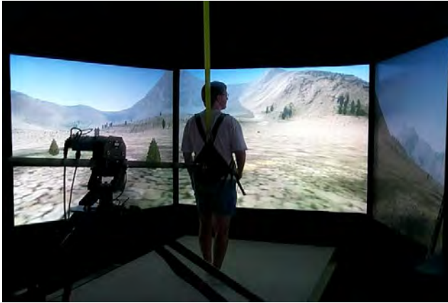
Figure 1: The mechanical tether of the Sarcos Treadport applies torso forces to a user via a harness worn by the user.
