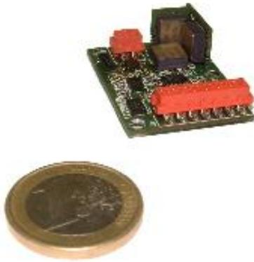
Fig. 2. Sensor provided by Technaid. This sensor is a combination of triaxial accelerometer, gyroscopes and magnetometer in order to provide six-degree-of-free dom motion estimation.
