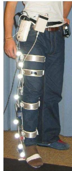
Fig. 5. Lower-limb exoskeleton for functional compensation of gait.
