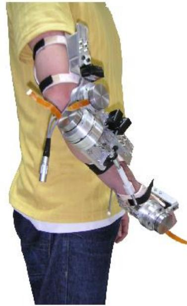
Fig. 1. WOTAS exoskeleton for tremor suppression.
