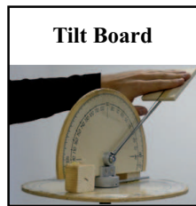
Figure 3. The tilt board allowed participants to haptically report the perceived tilt displayed by the human system interface.
