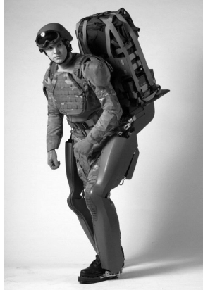
Fig. 24. One of the Berkeley Lower Extremity Exoskeleton Prototypes. The limbs are enclosed by plastic covers ( http://bleex.me.berkeley.edu/bleex.htm ).
