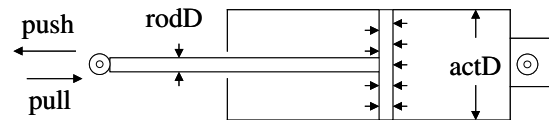
Fig. 15. Bi-directional linear hydraulic actuator schematic. Note that the area on which the internal pressure can act is different on the piston and rod sides of the actuator. This means that the actuator can push with more force than it can pull given the same supply pressure.
