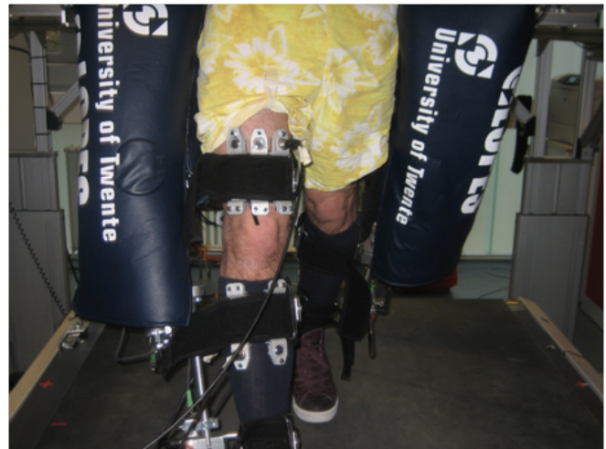
Fig. 4. First prototype of the sensorized belt during a gait rehabilitation task performed by the LOPES. In this example, the pressure is measured using six elements on the upper leg connection cuff (only three can be seen in this picture), and four (two visible) for the lower leg.
