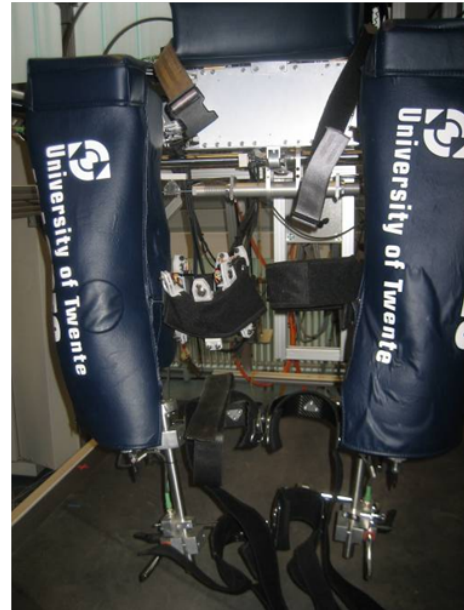
Fig. 1. The Lopes lower-limb rehabilitation exoskeleton, together with the sensorized fastening belts. In this example, only the right hip fastening point is sensorized with six pads (three in the front, and three in the rear of the belt).
