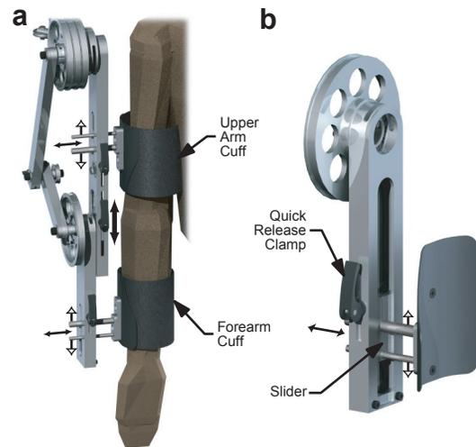
Fig. 5. (a) A CAD drawing illustrating the arm cuff attachments and adjustments. Each cuff has two translational adjustments to correctly align the limb segments relative to the mechanism structure: perpendicular to the link (small arrows) and parallel to the link (hollow arrows). A fifth adjustment (large arrow) moves the location of the elbow joint to change the length of the upper limb link. (b) A close-up of the cuff attachment, showing the quick-release clamp.
