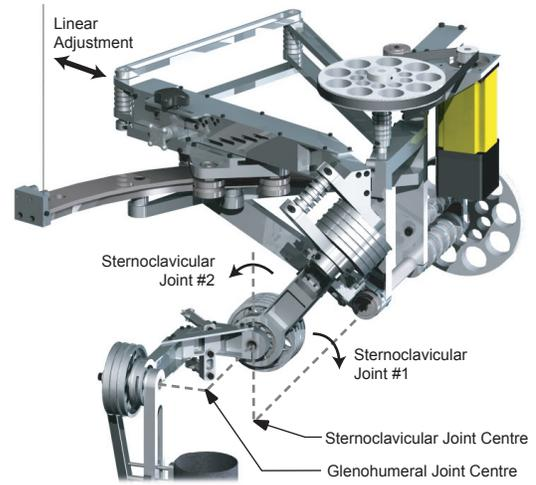
Fig. 4. A CAD drawing of the shoulder girdle mechanism. The two joint axes intersect at the user's sternoclavicular joint. The second joint is a translation along a curved track, producing a rotation about the vertical axis. The joint is driven by a hinged linkage system. A single linear adjustment shifts the entire shoulder/elbow mechanism to align the spherical joint with the user's glenohumeral joint centre.
