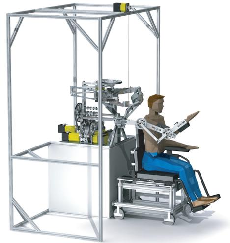
Fig. 1. MEDARM system consists of a 6DOF robotic exoskeleton mounted onto a support structure. The motors and electronics are mounted underneath the robot, and external gravity compensation is provided by a motorized vertical cabling system. A movable chair is used to bring the user into alignment with the system.
