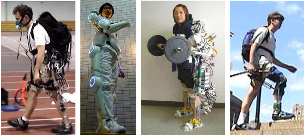
Fig. 5. MIT exoskeleton during metabolic testing [35], HAL-5 exoskeleton [41], nurse-assisting exoskeleton [43], and the RoboKnee [44]. Image credits (from left to right): Prof. Hugh Herr, Biomechanics Laboratory, MIT Media Lab, Cambridge, MA; Prof. Sankai, University of Tsukuba/CYBERDYNE, Inc., Tsukuba, Japan; Prof. Keijiyo Yamamoto, Kanagawa Institute of Technology, Atsugi, Japan; Dr. Jerry Pratt, Institute for Human and Machine Cognition, Pensacola, FL.
