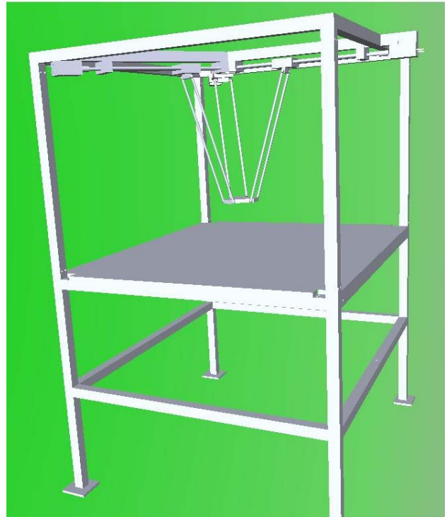
Fig. 7. TRIGLIDE Virtual Reality model made in Matlab/Simulink
