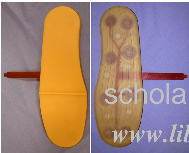
Fig. 7 Top (left) and bottom view of packaged sole. The bottom portion of the sole is semi-transparent and allows viewing of the flexible circuit board and electrical components.
