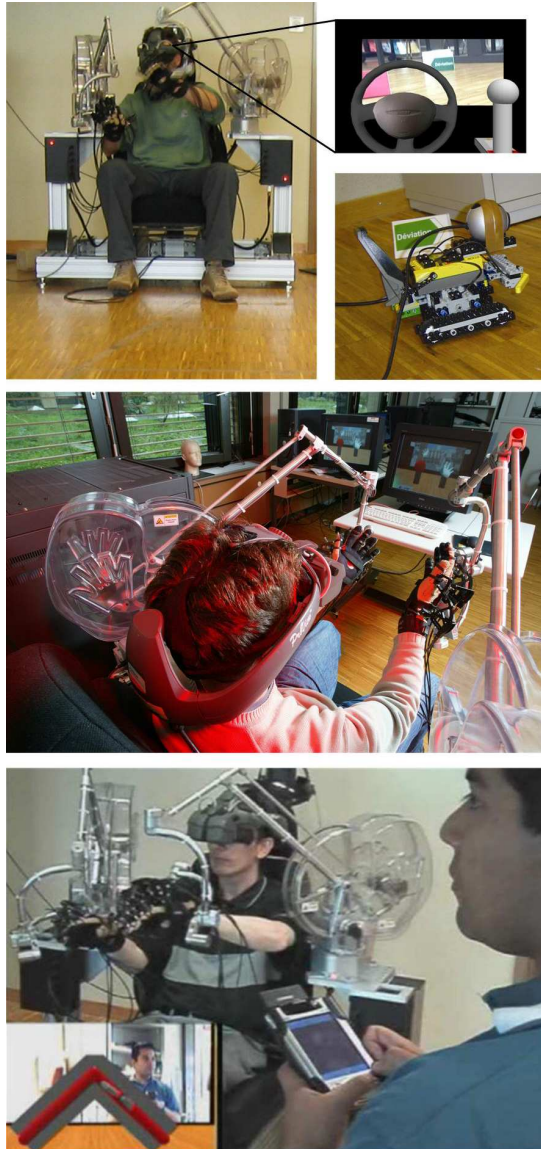
Figure 1. Research using a Haptic Workstation™. Top: teleoperation of robots; Middle: mediators, driving virtual vehicles; Bottom: telerehabilitation, kinesthetic therapy.
