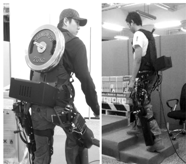
Fig. 9 Step Walking Test while Wearing the Lower Exoskeleton System with payload
