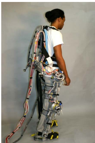
Figure 7: IHMC Mobility Assist Exoskeleton modified for straight line walking. The hip ab/adduction actuators and the hip internal/external passive rotation degrees of freedom have been replaced with a rigid link.
